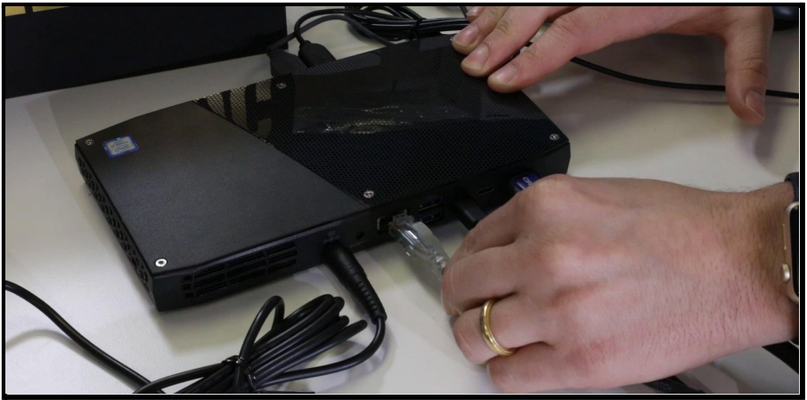
An Intel NUC i7 computer with a 256 GB SSD plugged into an ethernet LAN.
